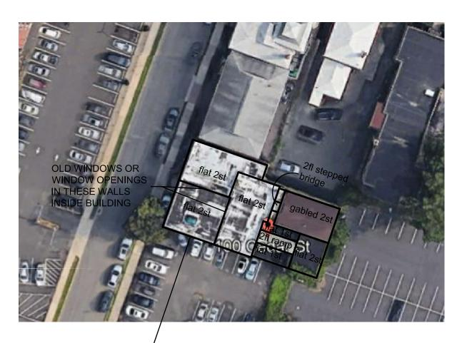
THIS SECTION APPEARS TO BE THE ORIGINAL BUILDING BASED ON INTERIOR WINDOW OPENINGS AND MAIN PASS DOOR. THE OTHER SECTIONS APPEAR TO BE ADDITIONS THAT WERE ADDED IN AN UNKNOWN ORDER.
