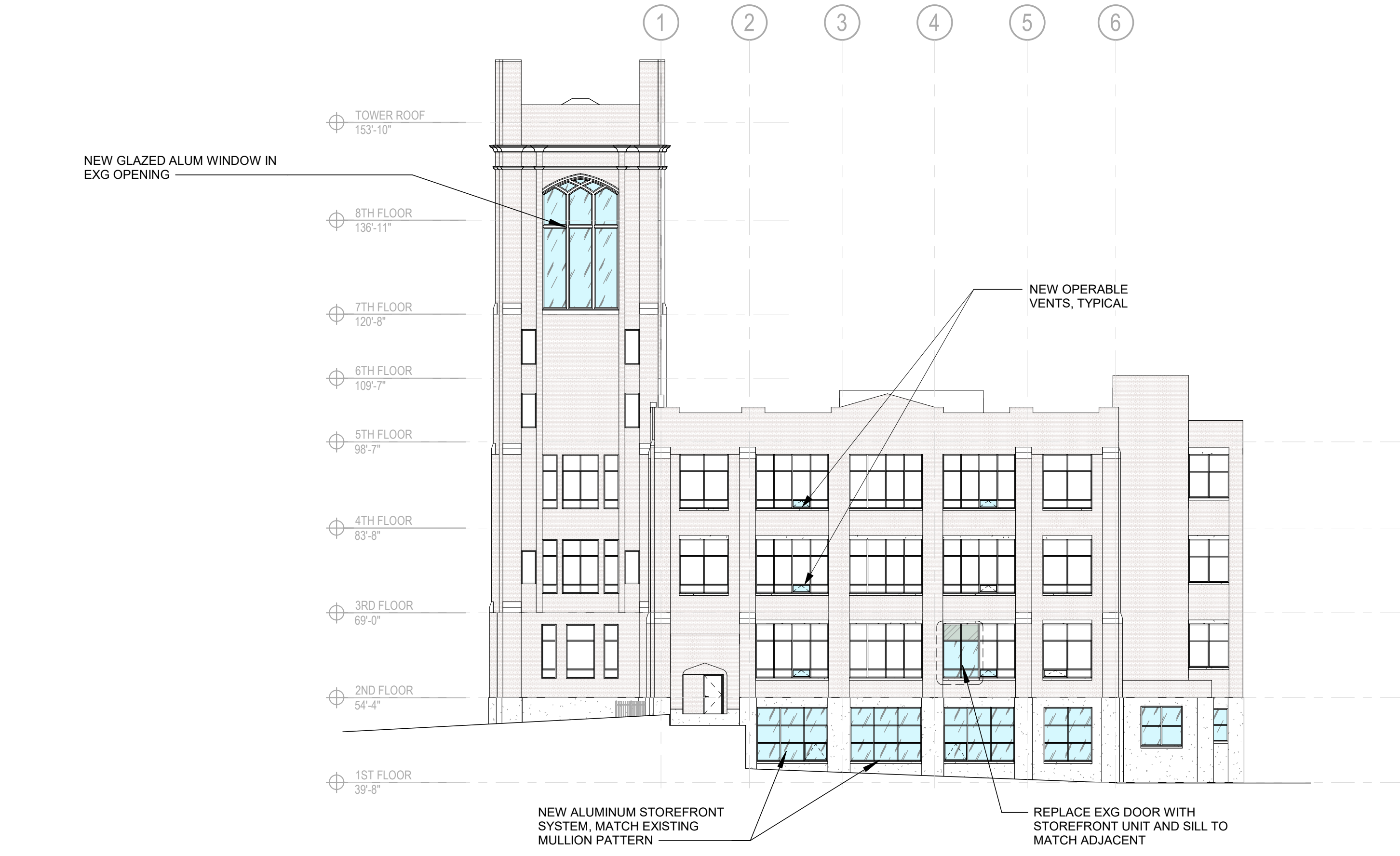
A3 SOUTH ELEVATION - NEW CONSTRUCTION EL-3 1/16" = 1'-0"
