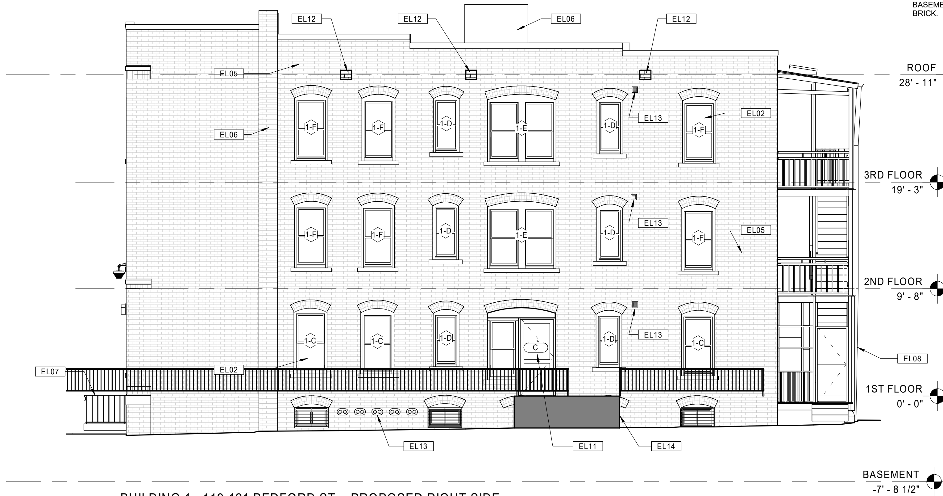
21 BUILDING 1 - 119-121 BEDFORD ST. - PROPOSED RIGHT SIDE ELEVATION Scale: 3/16" = 1'-0"
