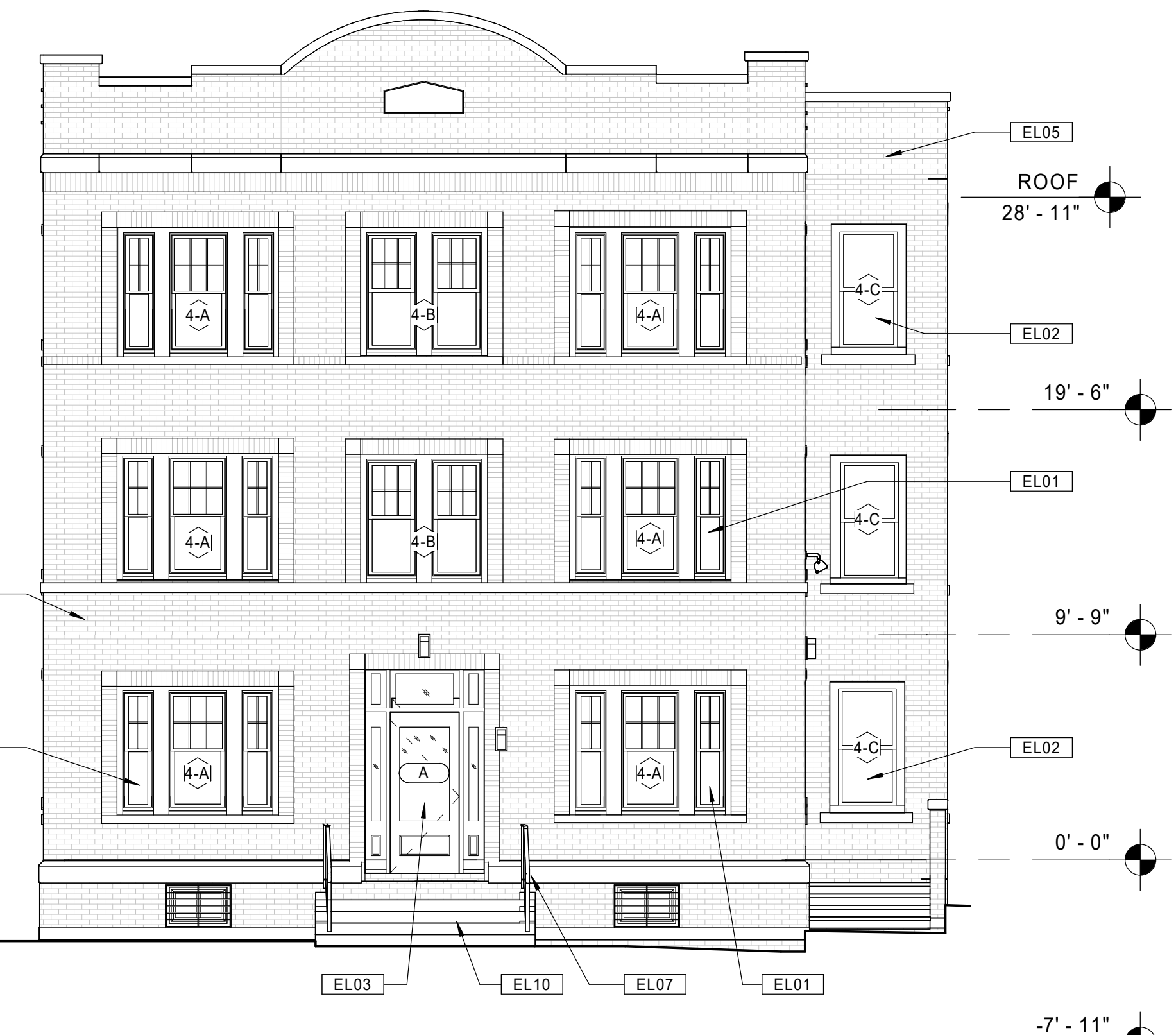
10 BUILDING 4 - 124-126 BEDFORD ST. - PROPOSED FRONT ELEVATION Scale: 3/16" = 1'-0"
