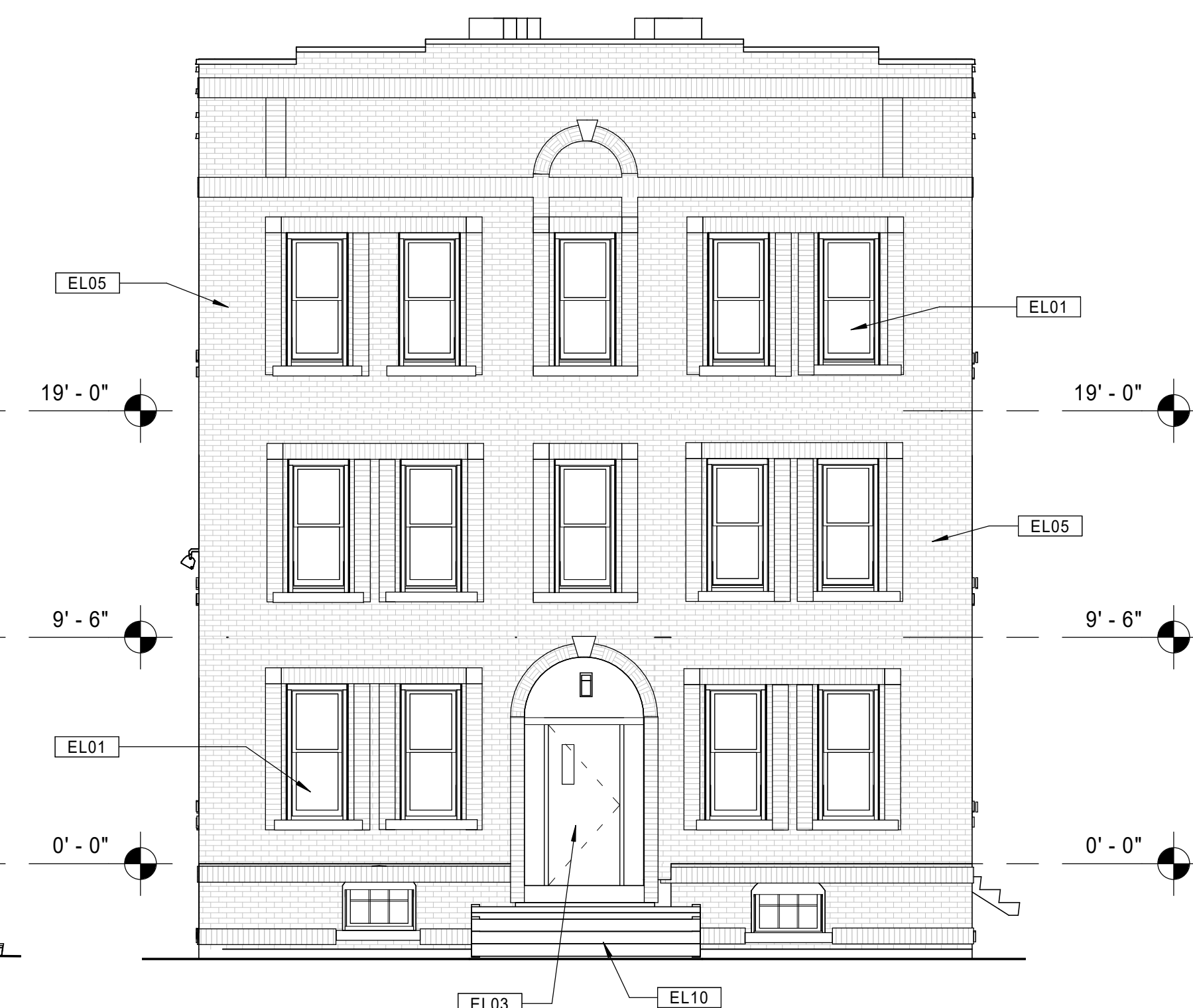
11 BUILDING 5 - 127-129 BEDFORD ST. - EXISTING REAR ELEVATION Scale: 3/16" = 1'-0"
