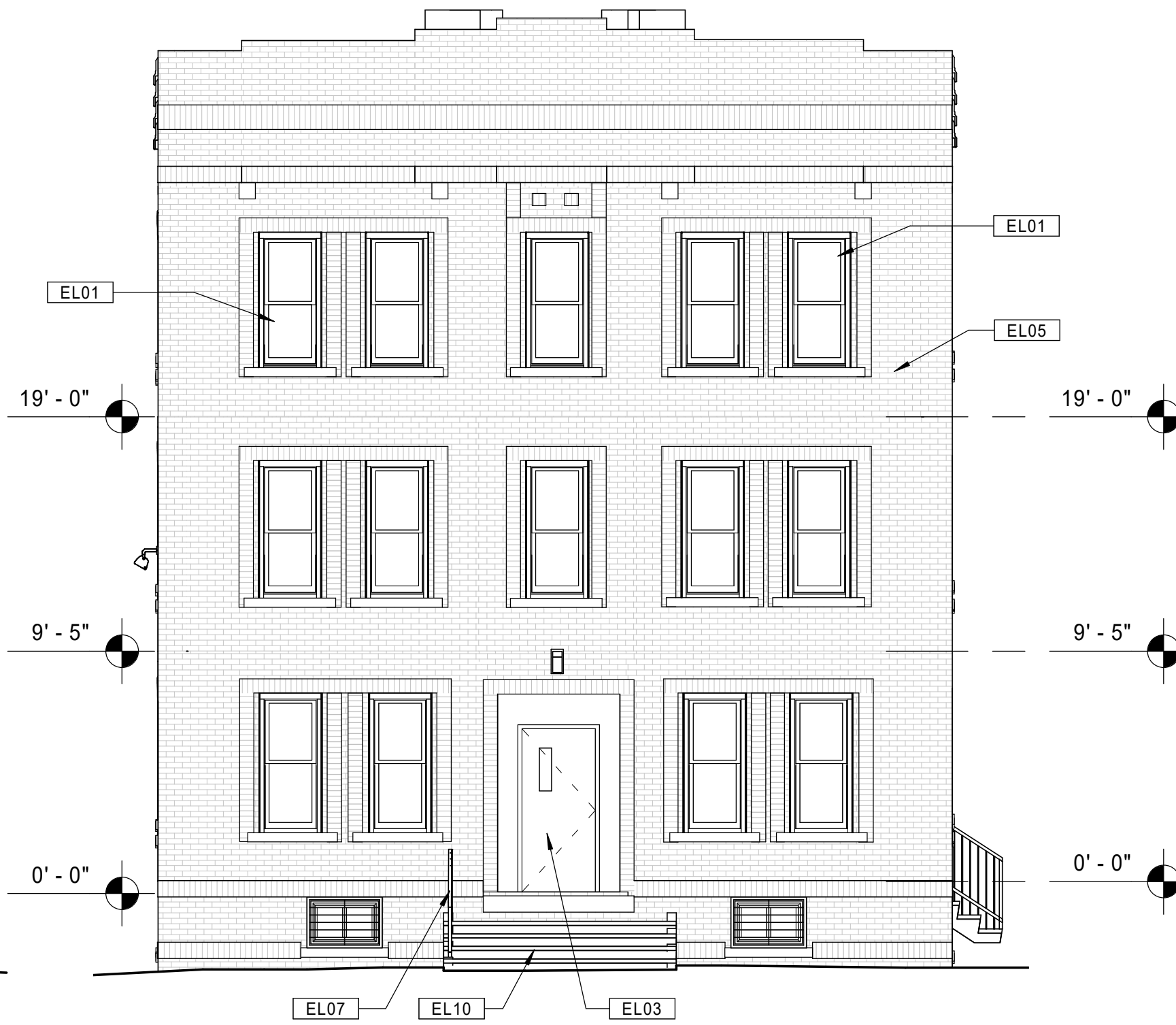
11 BUILDING 7 - 131-133 BEDFORD ST. - EXISTING REAR ELEVATION Scale: 3/16" = 1'-0"
