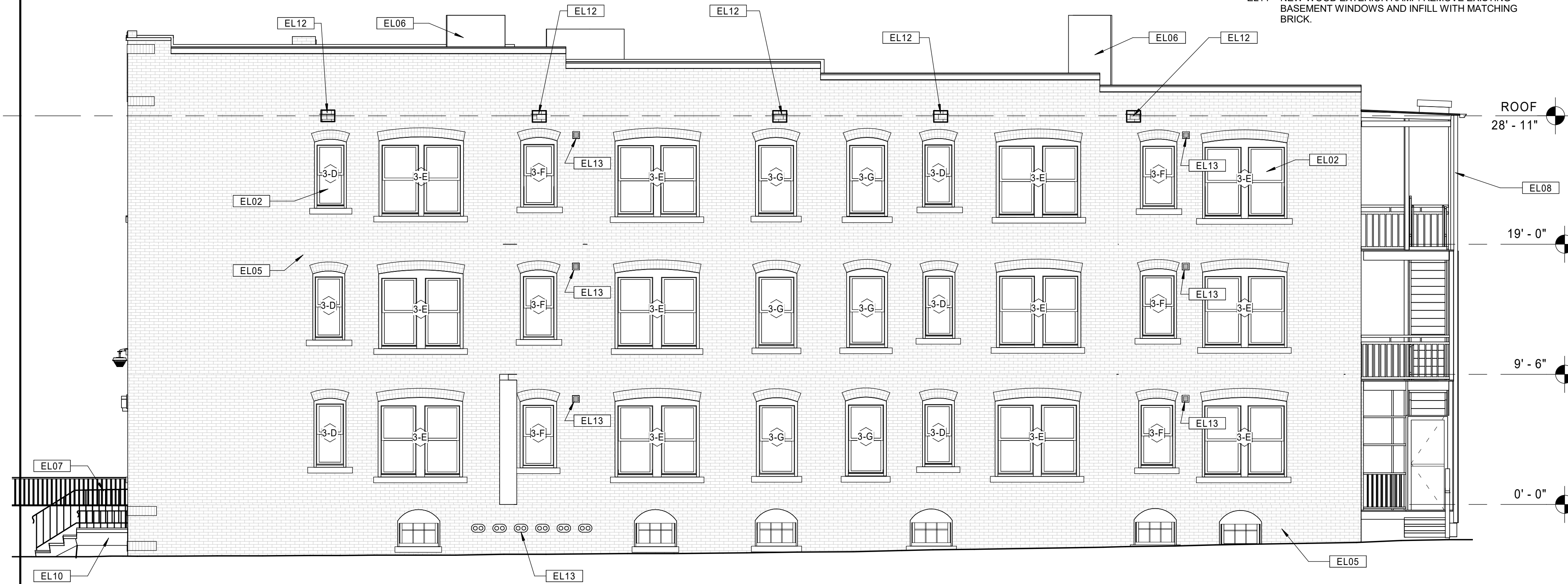
21 BUILDING 3 - 123-125 BEDFORD ST. - PROPOSED RIGHT SIDE ELEVATION Scale: 3/16" = 1'-0"
