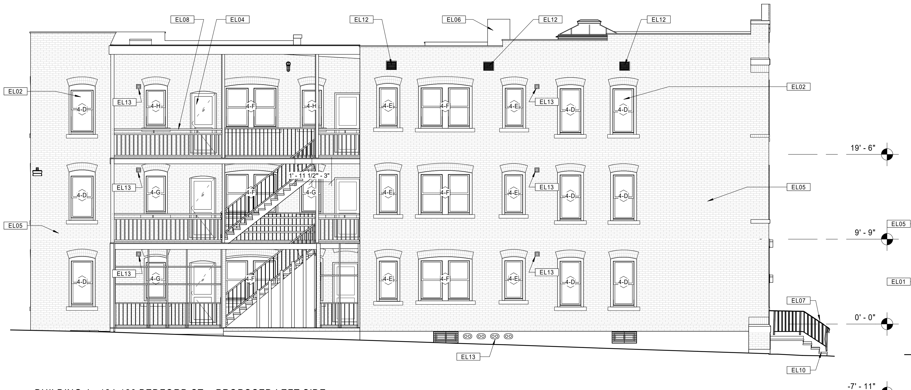
20 BUILDING 4 - 124-126 BEDFORD ST. - PROPOSED LEFT SIDE ELEVATION Scale: 3/16" = 1'-0"
