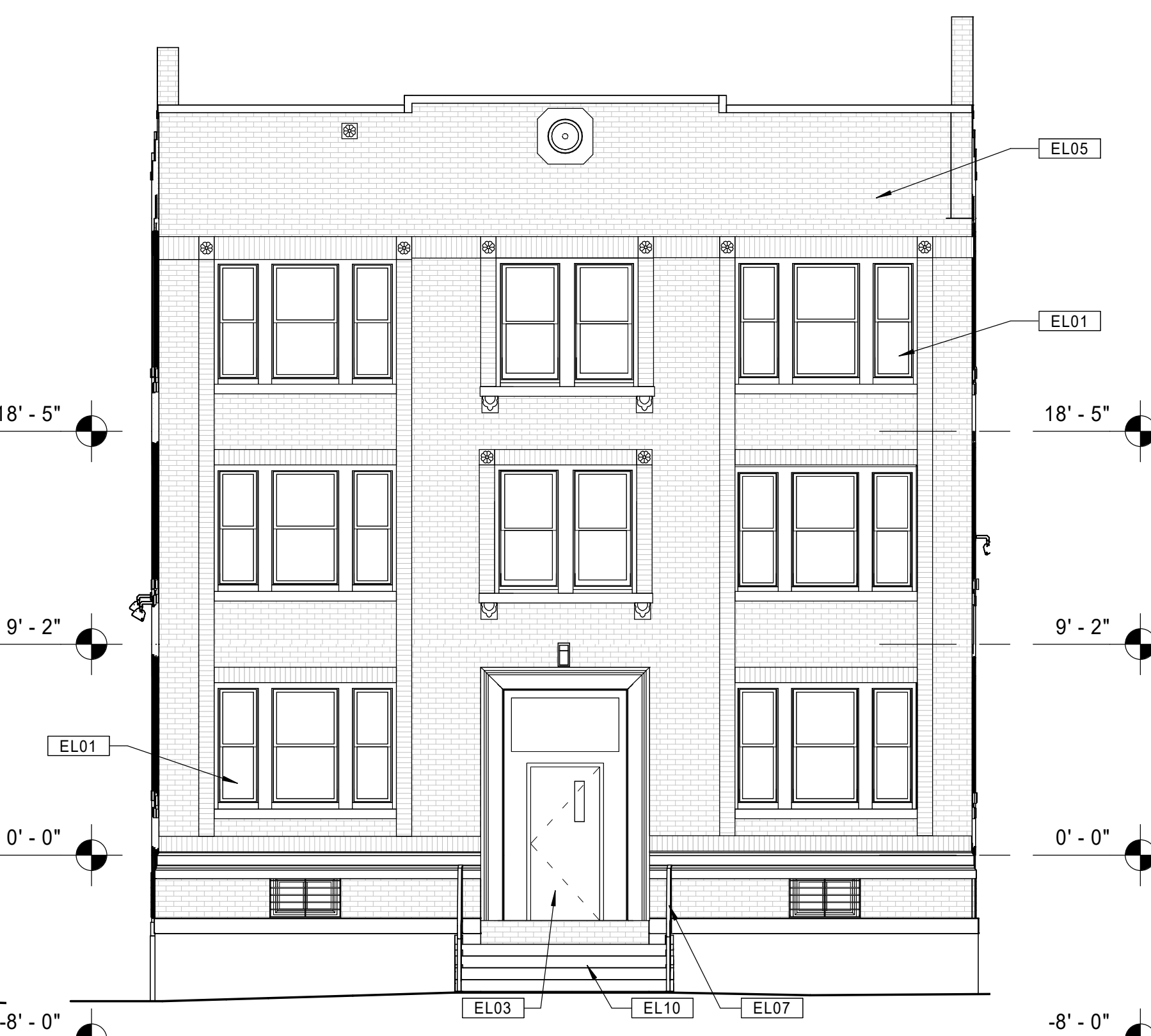
10 BUILDING 6 - 128-130 BEDFORD ST. - EXISTING FRONT ELEVATION Scale: 3/16" = 1'-0"
