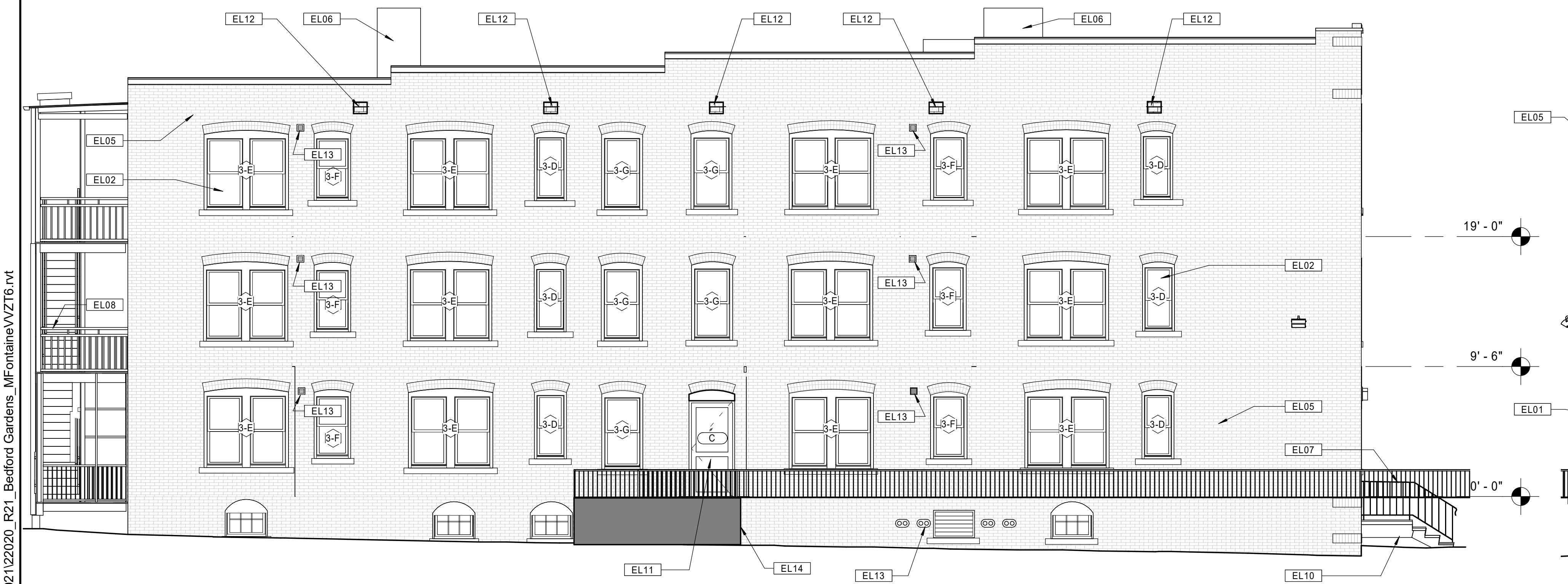
21 BUILDING 3 - 123-125 BEDFORD ST. - PROPOSED RIGHT SIDE ELEVATION Scale: 3/16" = 1'-0"
