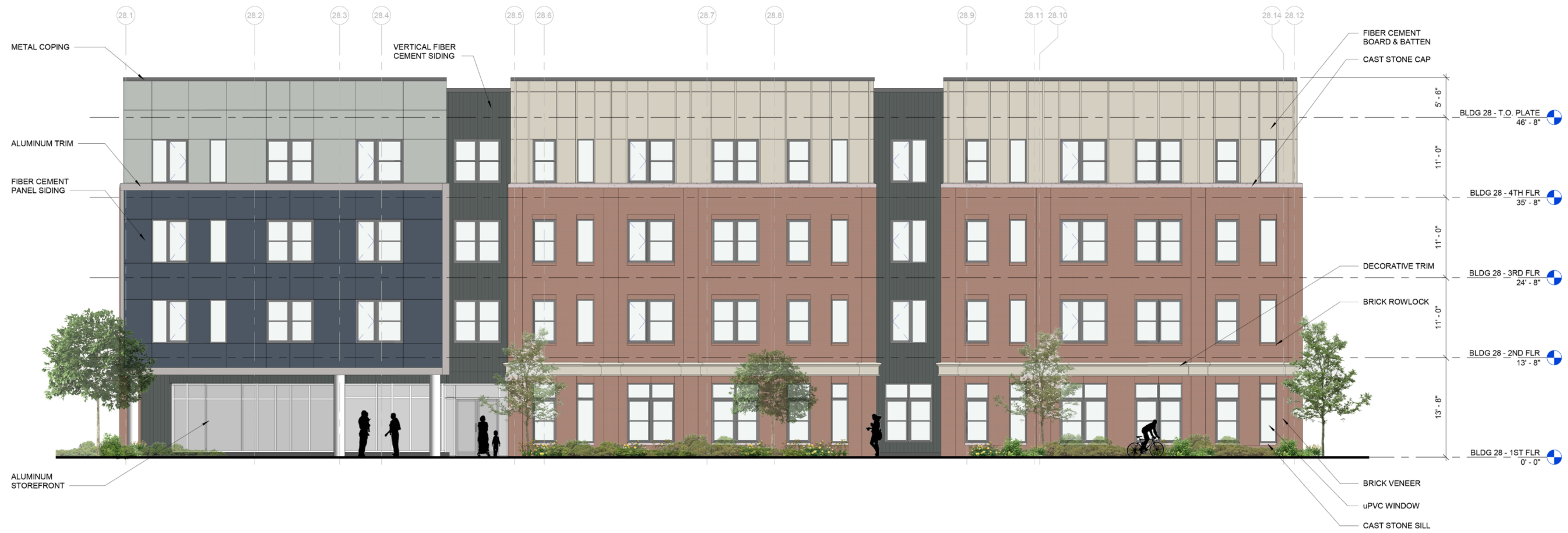
2 EAST ELEVATION - BLDG 28 1/8" = 1'-0"
