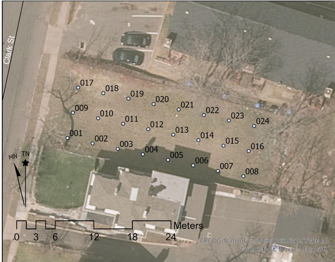
Figure A. Grid layout at the investigation site. Grid spacing is 3 meters by 3 meters.
